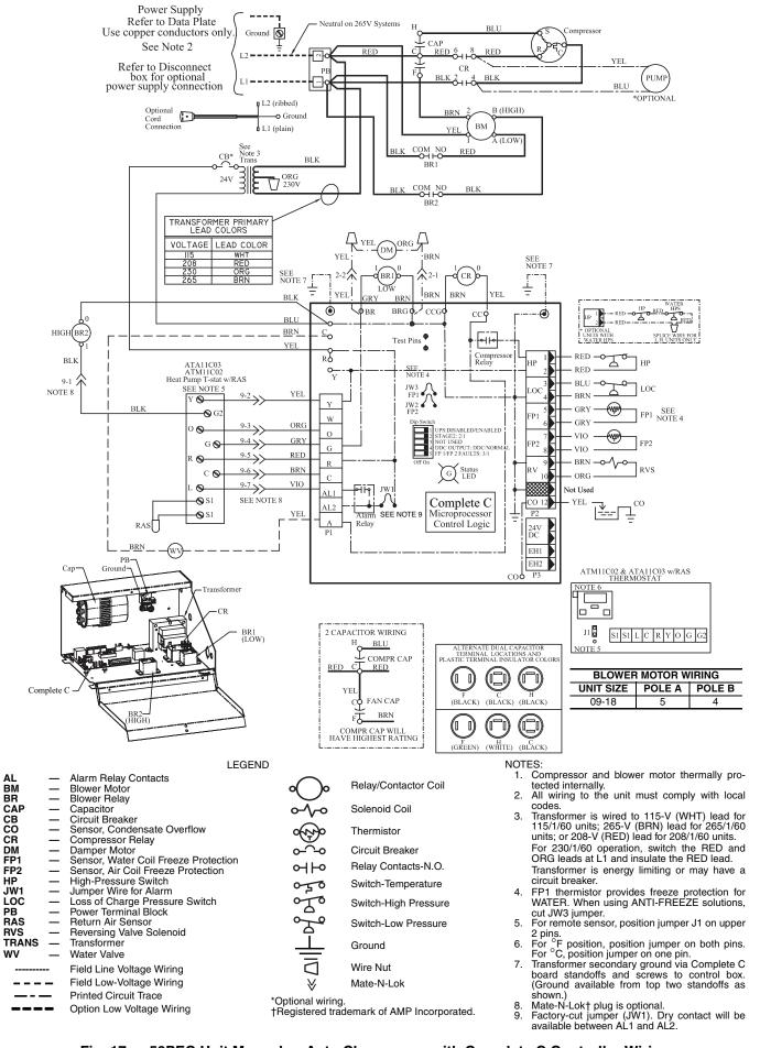
Fig. 17 — 50PEC Unit Manual or Auto Changeover with Complete C Controller Wiring
